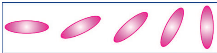
Figure 1: Combining varied shape, orientation, or diffusion angles on different areas of a single diffuser produces distinct patterns even when lit with one LED array.
