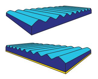
The Round-Tip pattern is embossed on a 10 mil polycarbonate substrate which has higher temperature durability when compared to polyester films. The RTD film is available with or without an integrated diffuser on the back. The combined RTD film and diffuser reduces the number of films in the display stack.
